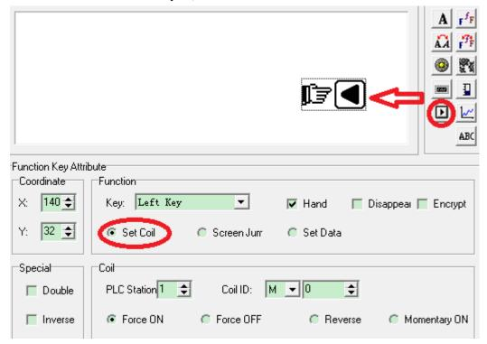
Force ON: set ON the auxiliary relay Force OFF: set OFF the auxiliary relay
