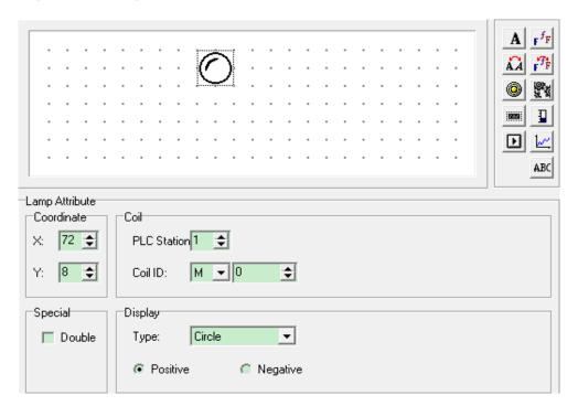
> PLC station PLC station no. communicating with OP panel
