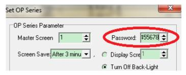
Set the password as you need (no max limit for the password). This password is for all encrypt buttons. User has to input correct password to operate the encrypt buttons.
