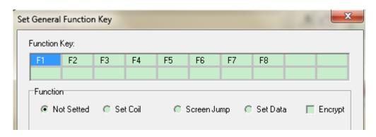
Function key includes eight keys (F1~F8). Each key has 4 functions(not setted/set coil/screen jump/set data) which can be used together with encrypt function.
