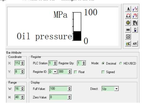
This application will monitor the value of register D300. For example: when D300=100, the bar shows the full scale, D300=50, the bar shows the half scale.
