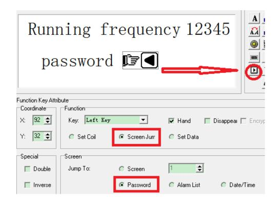
When user press SET button on the OP panel, the register cannot be operated. User has to press left key to enter password window.
