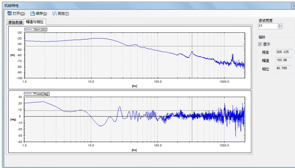
5. set the filter width (to see resonance frequencies clearly), find the resonance frequency;
