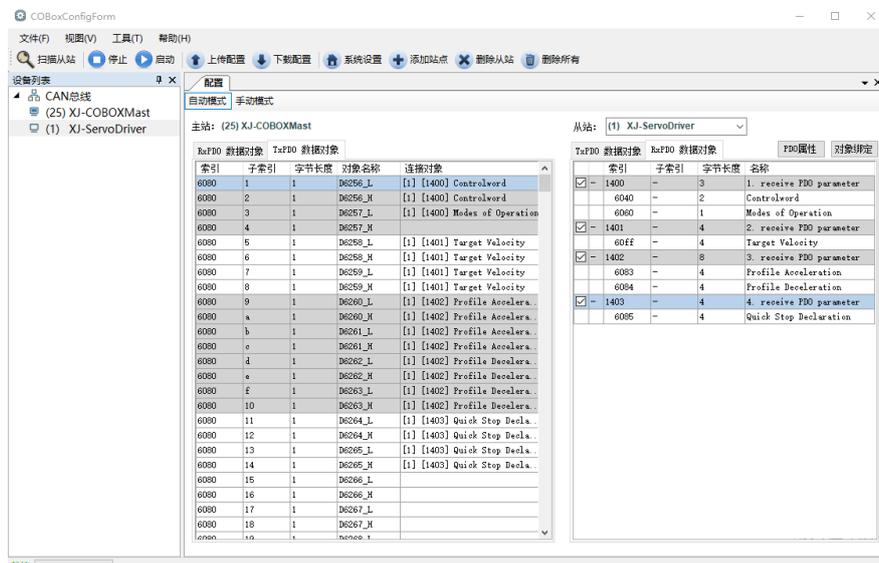
② Download and activate the configurations. The slave station state machine automatically switches from PreOP to OP state. At this time, SDO and PDO can receive and send signals. The mapping of object dictionary can be monitored or modified through XDPpro. The specific correspondence is shown in the figure below.
